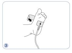
Wrap the sensor around the site, without stretching the tape, so the optical components directly oppose each other. Anchor the cable with a piece of medical-grade tape. Plug the connector end of the sensor cable into the patient cable attached to the monitor.
