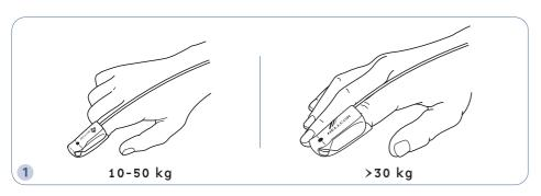
An index finger is the preferred sensor site. Alternatively, apply the sensor to a smaller finger, thumb or great toe. Use the pediatric sensor for pediatric patients weighing 10 to 50 kg. Use the adult sensor for adults weighing more than 30 kg.
